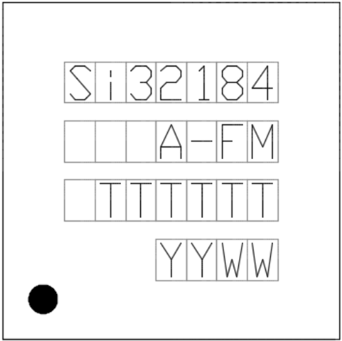
Figure 10.2. 40-Pin QFN Top Marking
