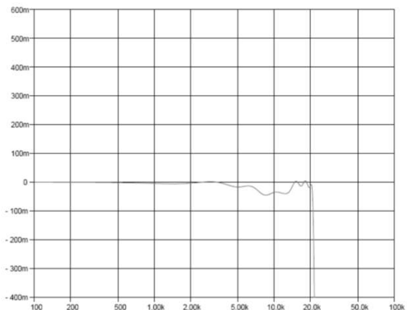
Figure 12: DAC Pass Band Attenuation (Audio Mode, 48 kHz)
