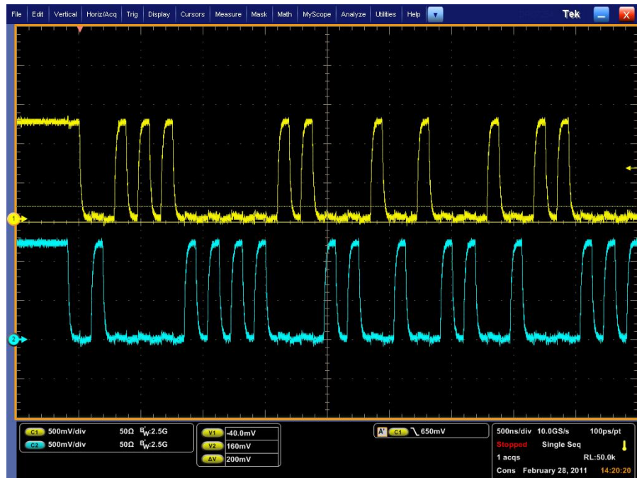
Figure 5. EMI4193 MIPI D-PHY LP Mode Measured Results
