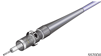
Figure 40 Screwing on the basic unit (with the example of an F-SMA connector)
