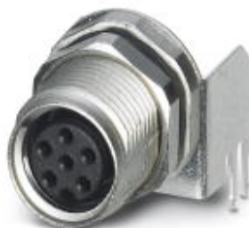
Sensor/actuator flush-type plug-in connector, socket, 6-pos., M8, rear/screw mounting with M10 fastening thread, with angled solder connection
