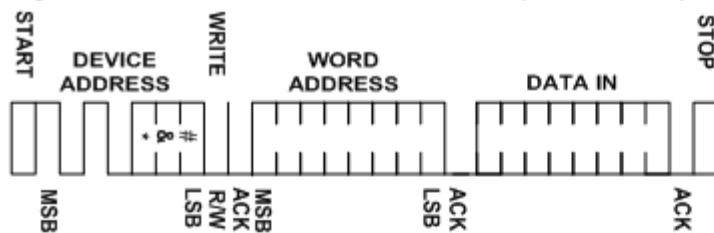
Figure 3: BYTE WRITE INSTURCTION (SDA INPUT)
