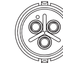
3 POSITION #16 PIN & SOCKET CONTACT
