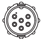
6 POSITION #20 PIN & SOCKET CONTACT
