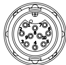
10 POSITION #22 PIN & SOCKET CONTACT
