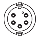
5 POSITION #20 PIN & SOCKET CONTACT
