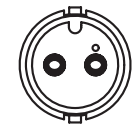
2 POSITION #16 PIN & SOCKET CONTACT
