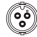
3 POSITION #16 PIN & SOCKET CONTACT
